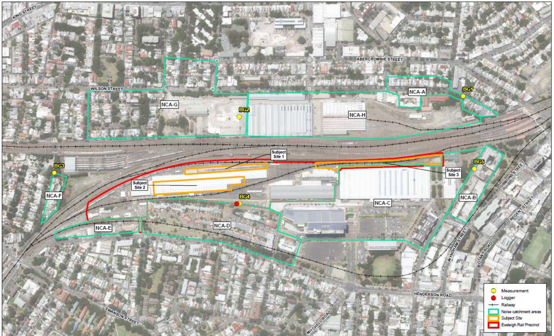
New Intercity Fleet Eveleigh Figure 7.1 Noise catchment areas and noise monitoring locations
