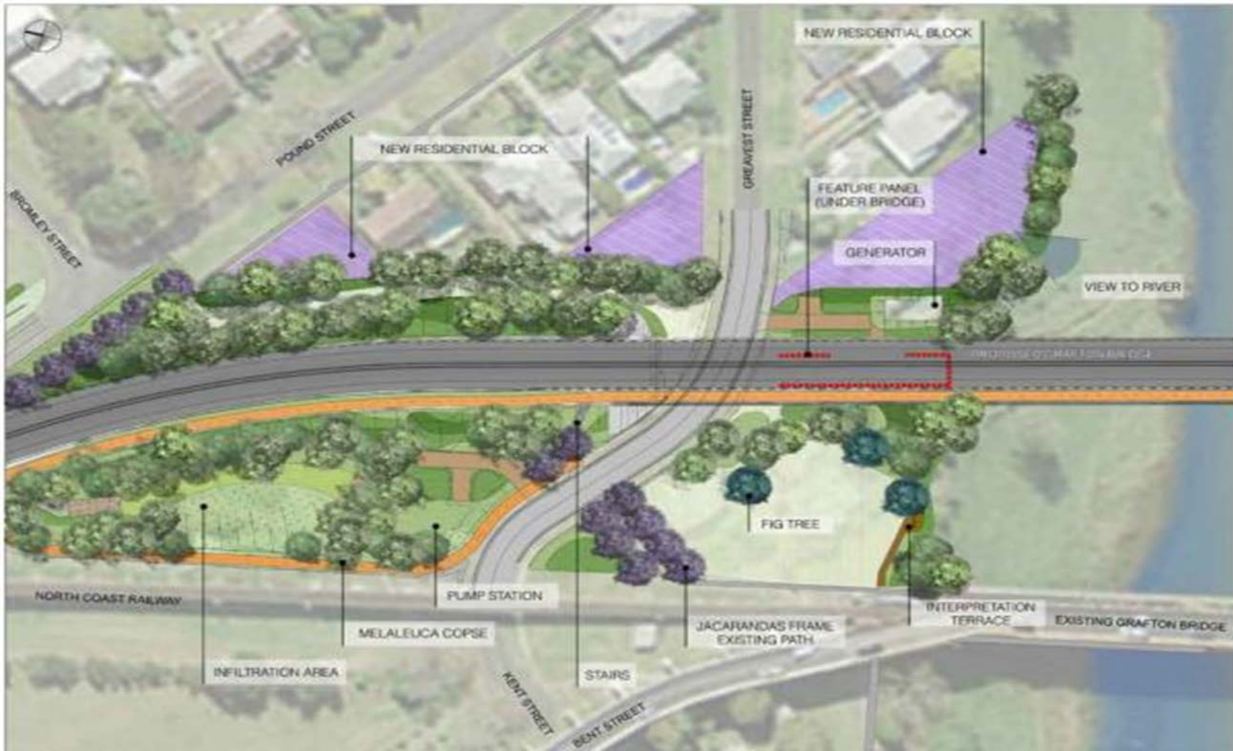
Fig. 5-37: Revised Greaves Street Precinct plan showing additional housing blocks, infiltration area under bridge and relocation of pump station and generator to improve overall outcome.
