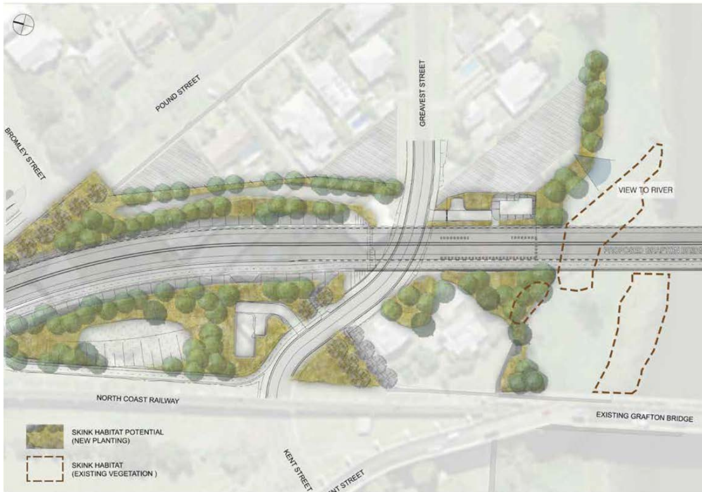
Figure 4. Landscaped areas where the microhabitat requirements of the Snake-toothed Three-toed Skink have been incorporated into the design. An additional 0.21 ha riparian vegetation will be planted within the existing skink habitat area shown here as a dashed line.
