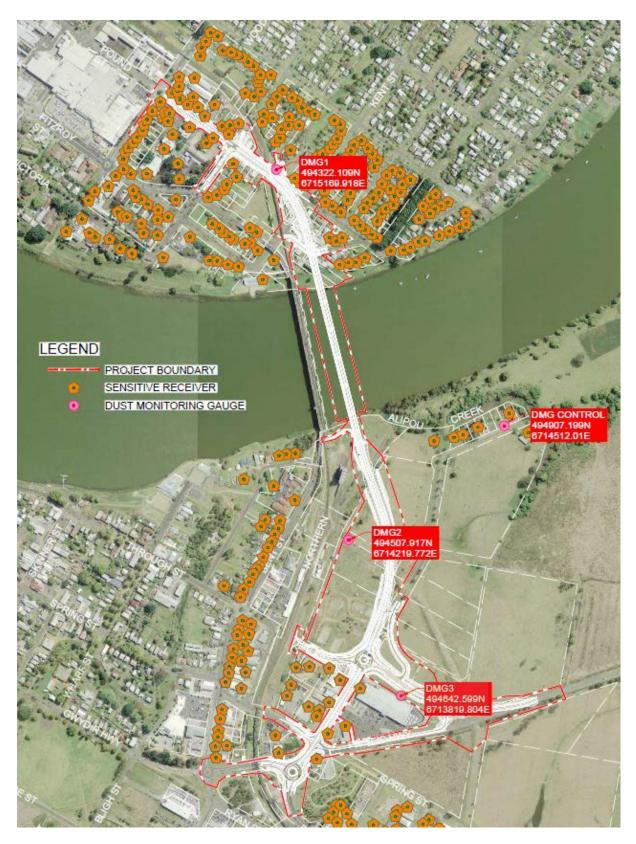
Figure A-1 Map showing indicative locations of dust monitoring gauges
