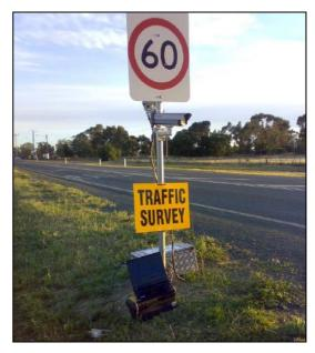
Above: Video camera technology set up on the roadside to capture passing vehicles.
