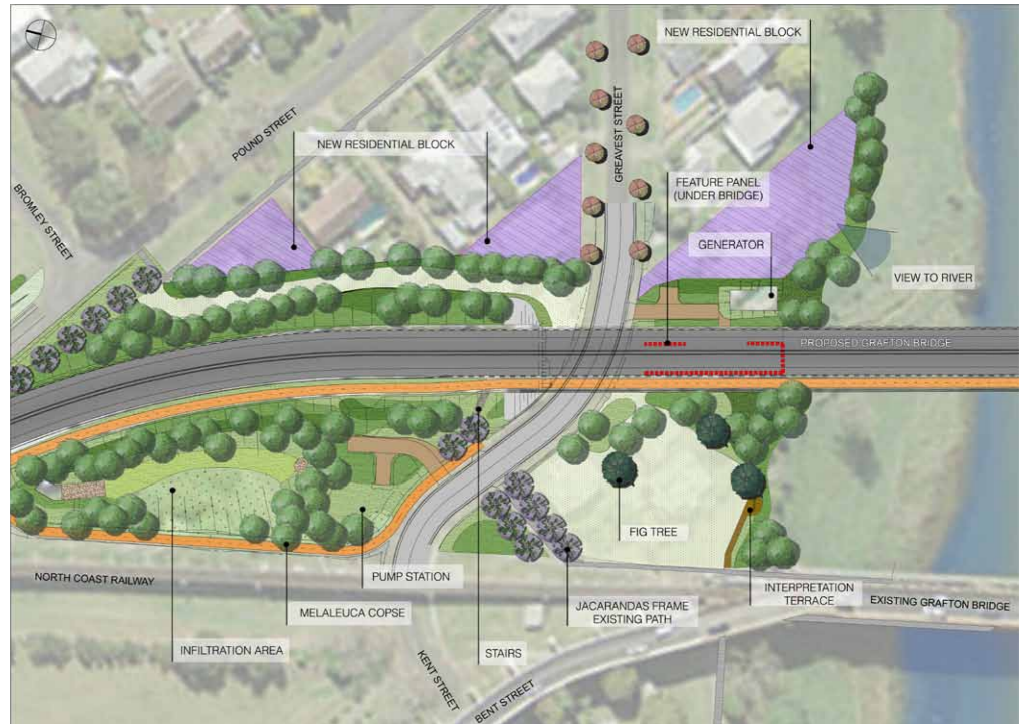
Fig. 5-37: Revised Greaves Street Precinct plan showing additional housing blocks, infill to under bridge and relocation of pump station and generator to improve overall outcome.
