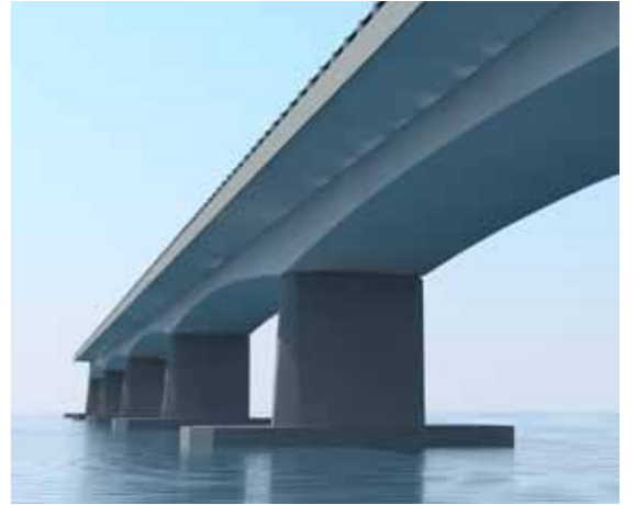
Fig. 4-17: Preferred bridge pier form
