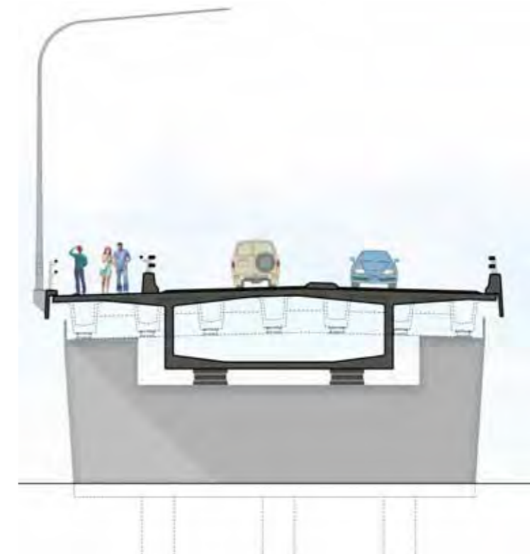
Fig. 5-55: Additional bridge over Clarence River at Grafton - Shows transition pier at South Grafton (Scale: 1:200)
