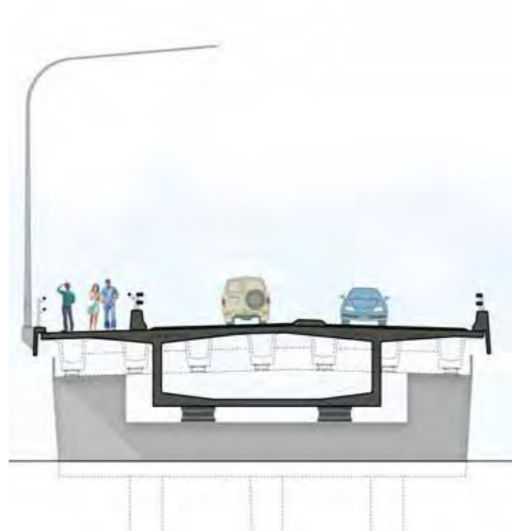
Fig. 5-53: Additional bridge over Clarence River at Grafton - Shows transition pier at Grafton near Greaves Street (Scale: 1:200)
