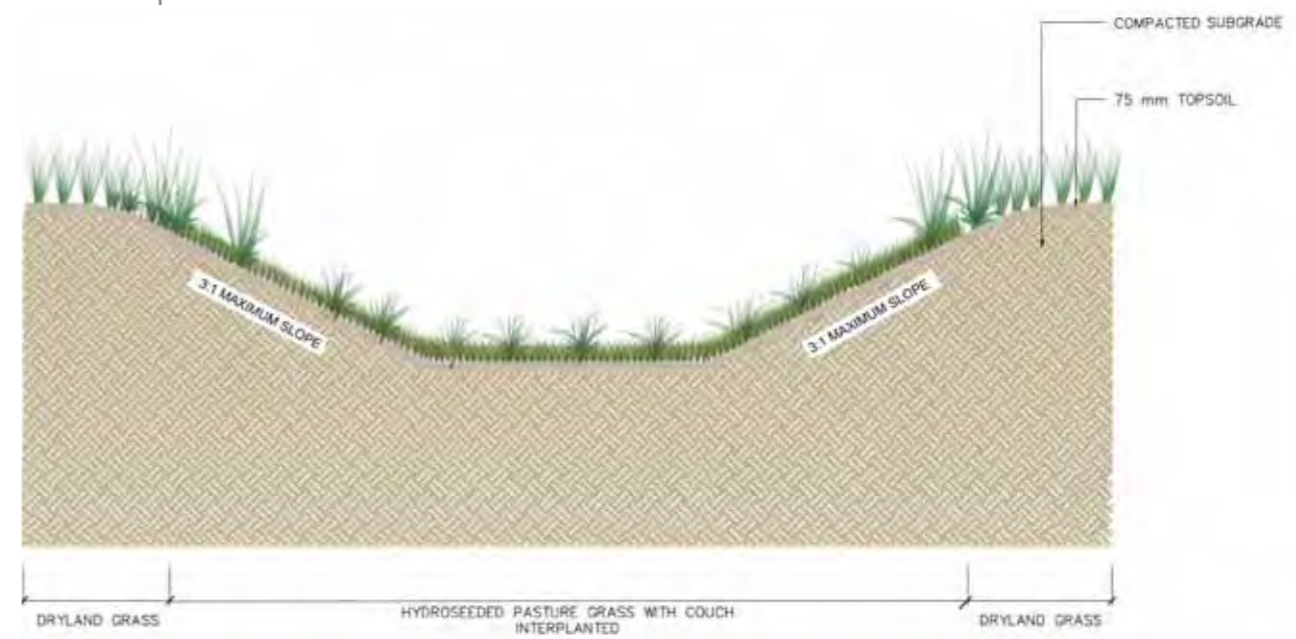
Fig. 6-29: Spill containment basin
