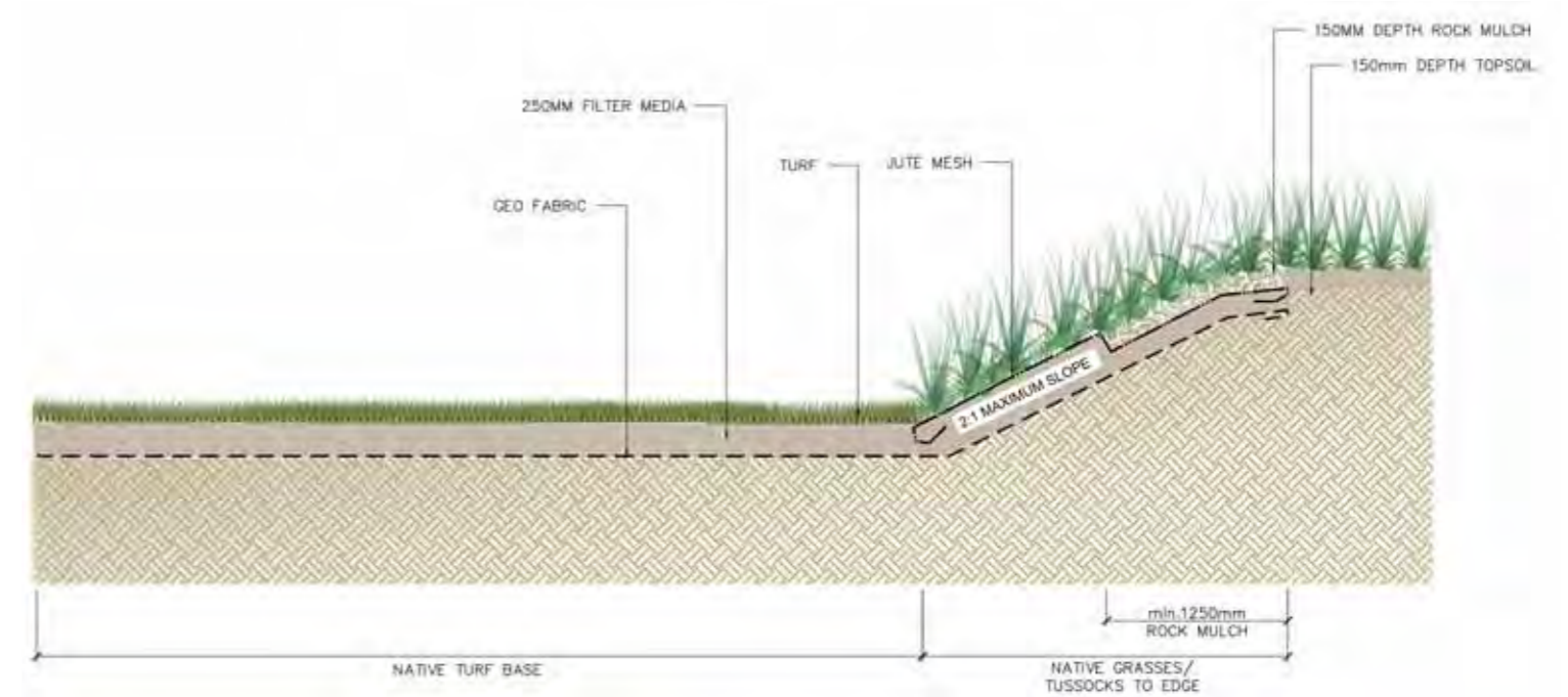
Fig. 6-28: Multi-purpose infiltration area - typical edge section
