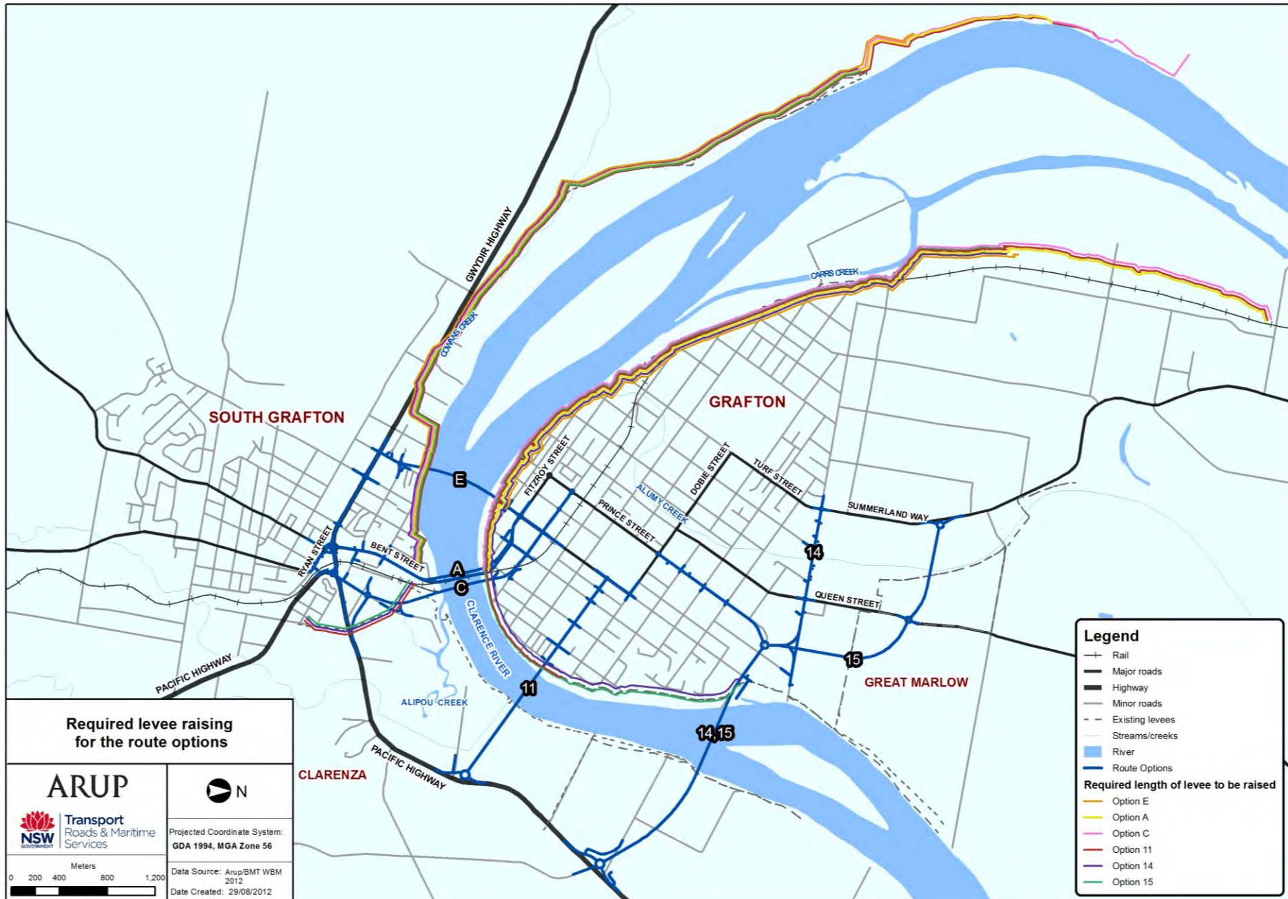
Figure 46: Required levee raising for the route options
