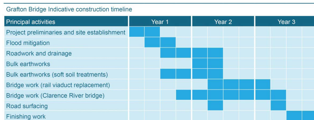
Figure 24: Grafton Bridge project indicative construction timeline
