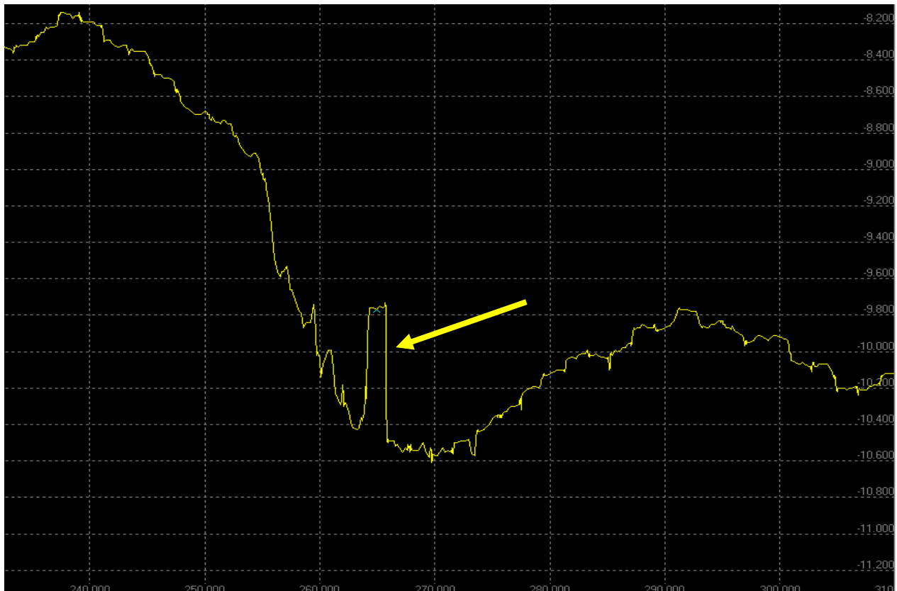
Figure 4:– Feature 1 -Clear bathymetric anomaly in the SBES data (yellow arrow), 1-2m length 0.8m height above the riverbed.
