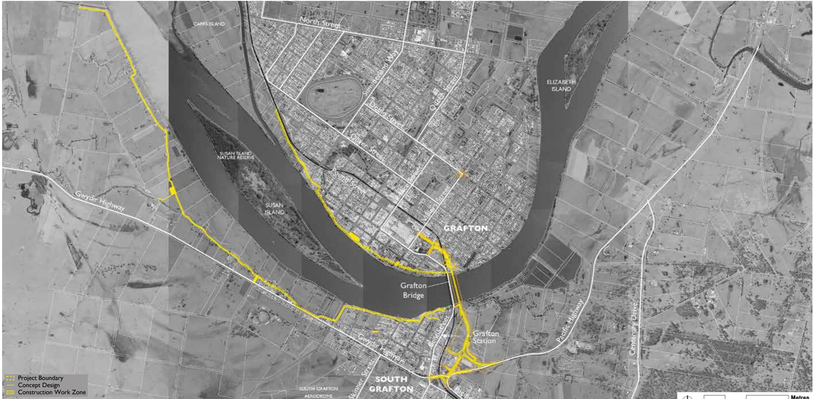
Figure 3.1: Extent of the proposed bridge, approach roads and levee upgrade works required to complete the project.
