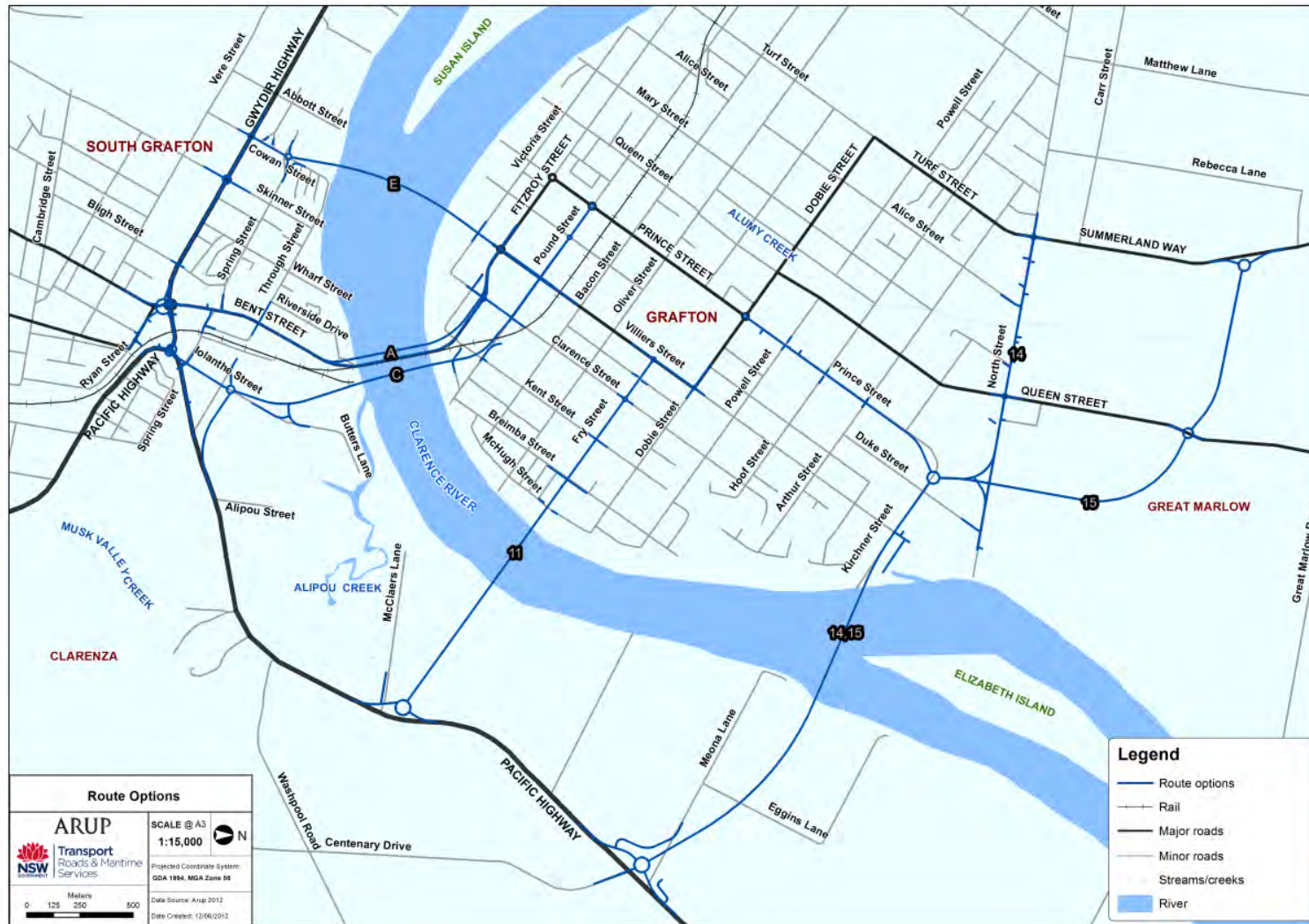
Figure 1: Short-list of route options for an additional crossing of the Clarence River at Grafton
