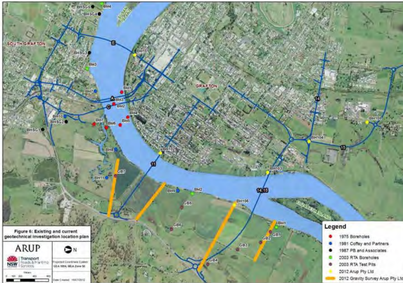
Figure 6 Existing and Current Geotechnical Investigation Location Plan
