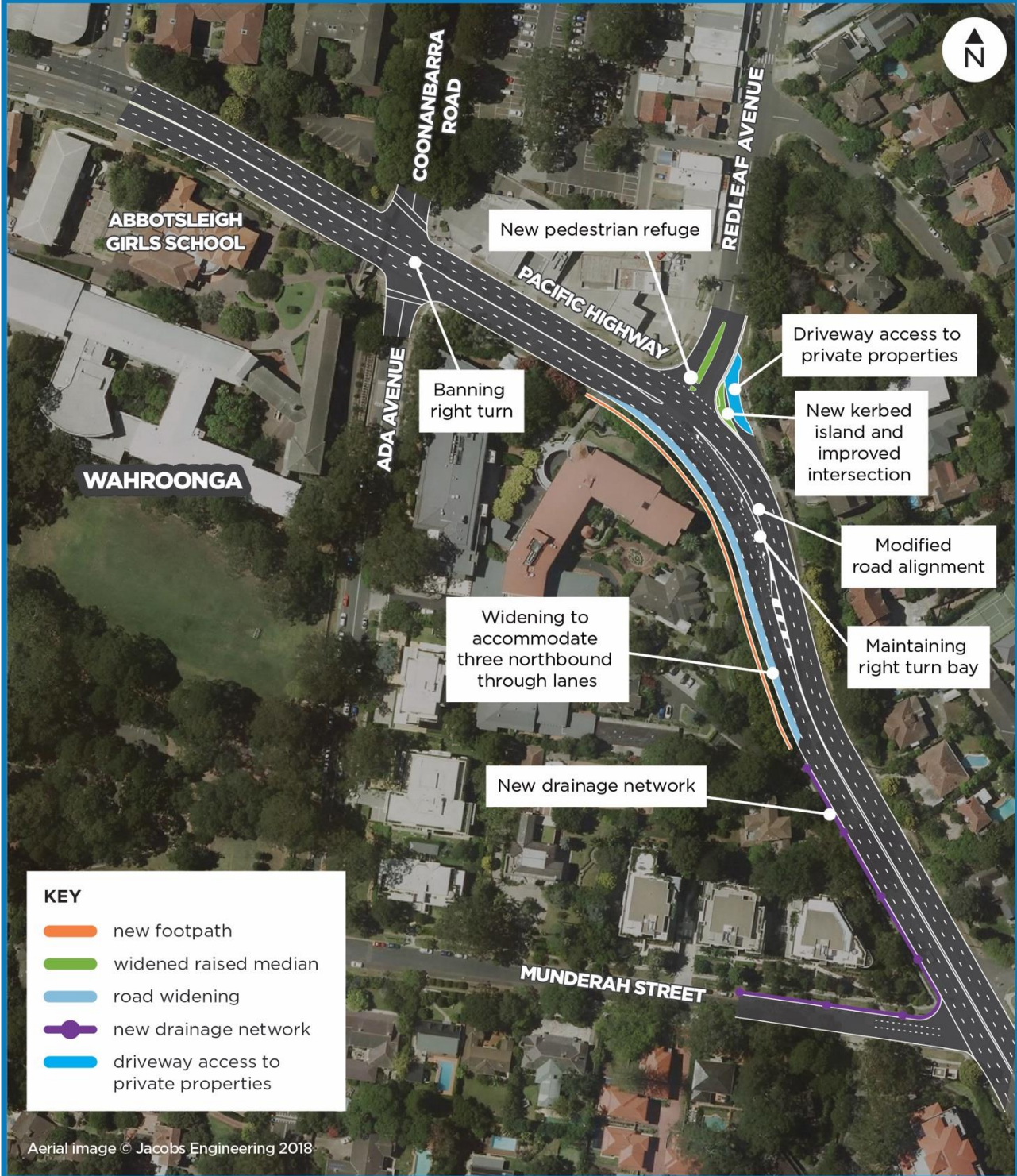
Figure 2: Proposed intersection upgrades on Pacific Highway at Coonanbarra Road and Redleaf Avenue, Wahroonga
