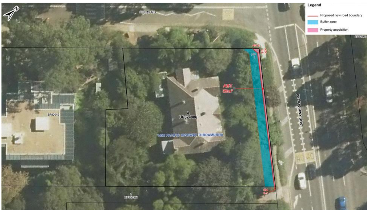
Figure 35 Area of Dwelling House site impacted by the proposed works of Pacific Highway at Finlay Road, Warrawee/Turrumurra
