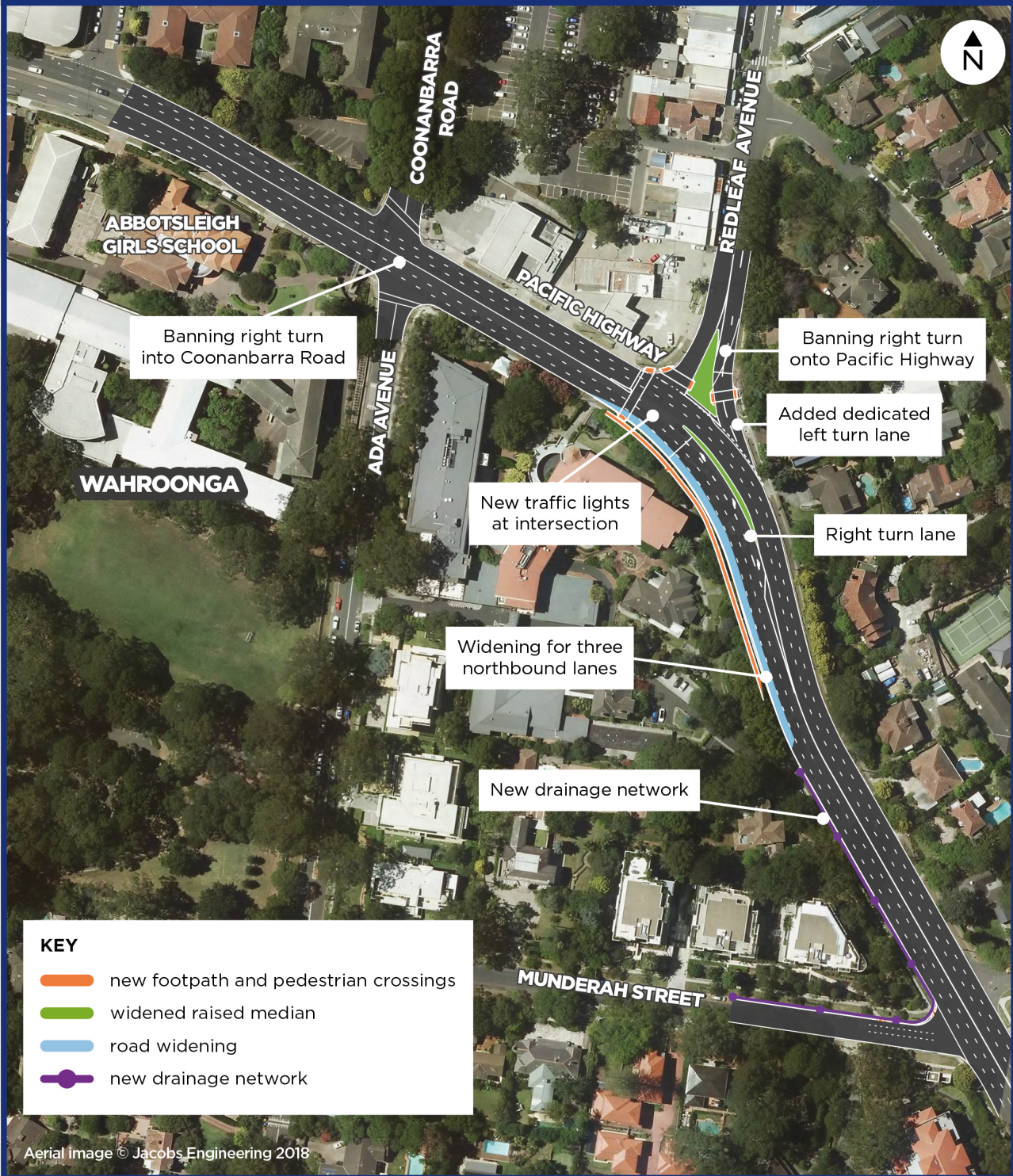
Figure 1-1: Main features of the proposal: Pacific Highway at Coonanbarra Road and Redleaf Avenue, Wahroonga
