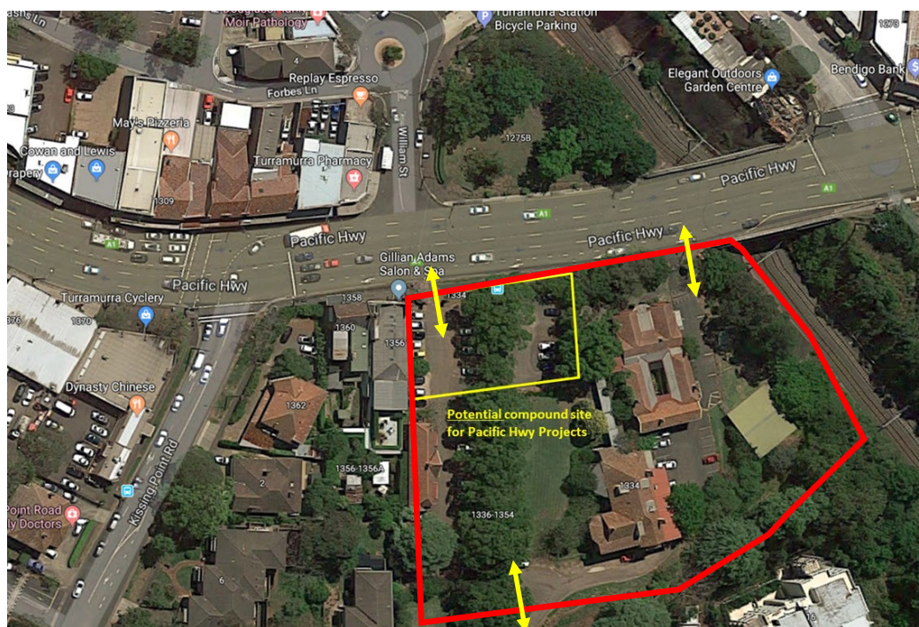
Figure 3-8: Proposed compound site location for the proposal – 1334-1354 Pacific Highway, Turramurra (extent of compound laydown area outlined in red, main compound area activities would occur within the main carpark area outlined in yellow, potential access points shown in yellow)
