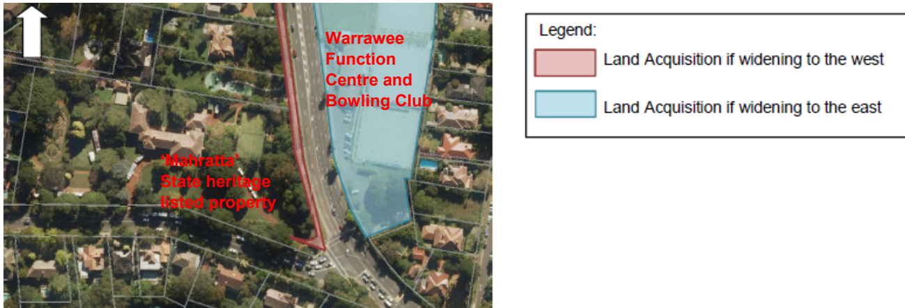
Figure 2-3: Potential land acquisition associated with widening to the east vs west near Fox Valley Road
