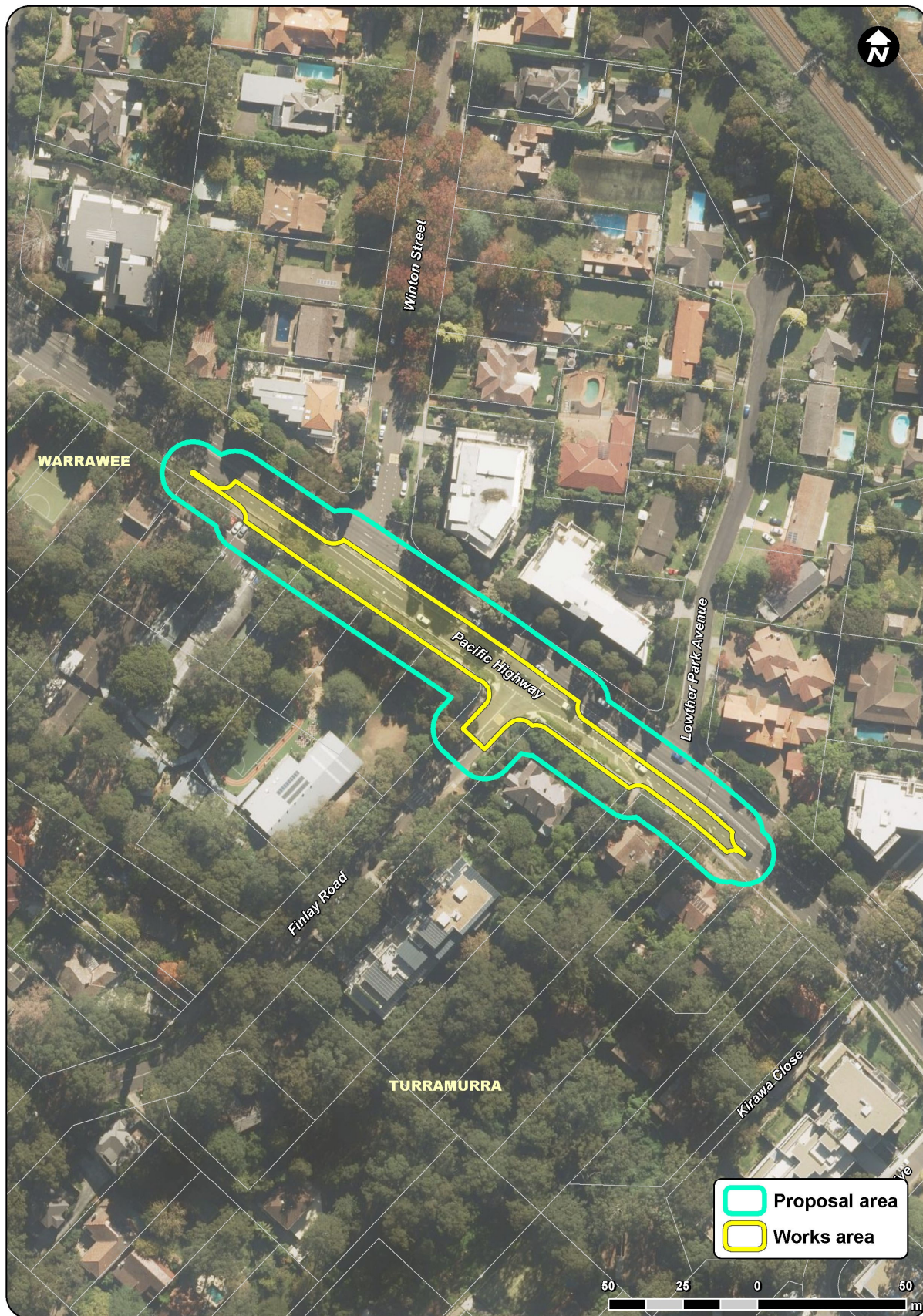
Figure 1-4: Proposal area / works area for Intersection 1 – Pacific Highway at Finlay Road, Warrawee/Turramurra (proposal area applies a 10 metre buffer either side of the works area zone)
