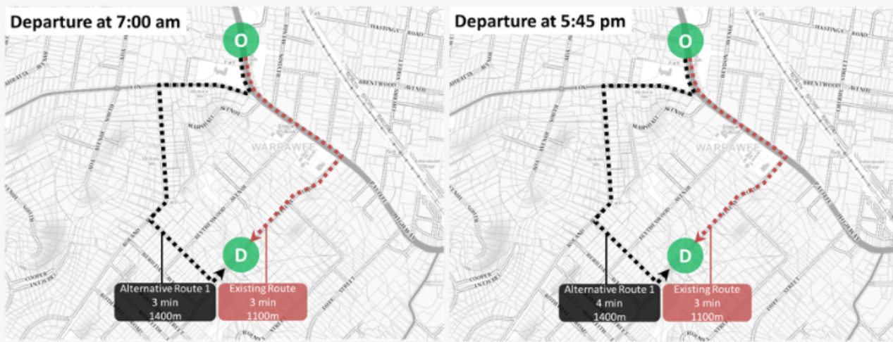
Figure 3-8: Proposed diversion routes as a result of the right-turn bans at Finlay Road, Warrabee/Turrumurra
