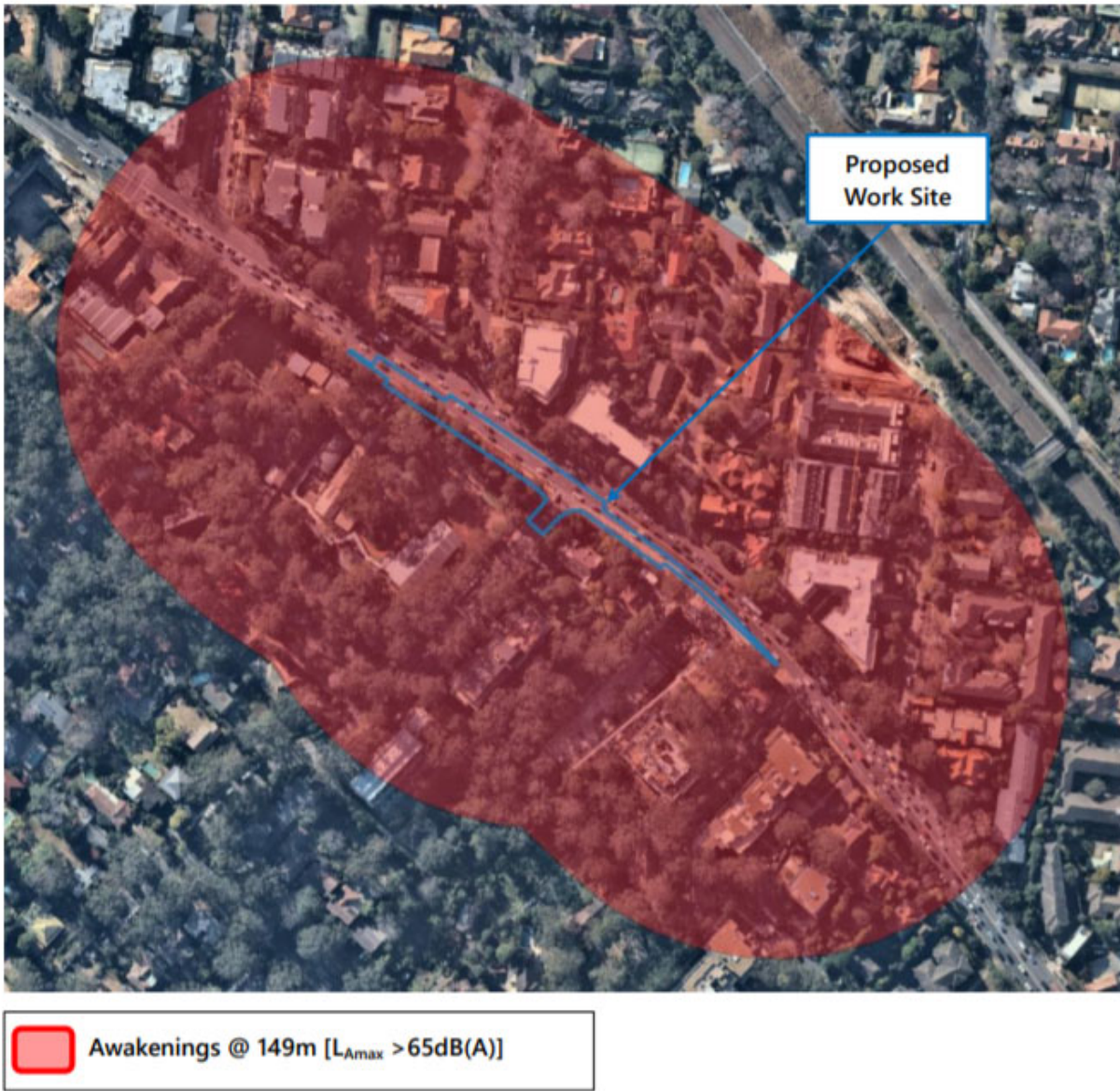
Figure 6-45: Site 1 / Intersection 1 – areas potentially impacted by maximum noise levels due to roadworks
