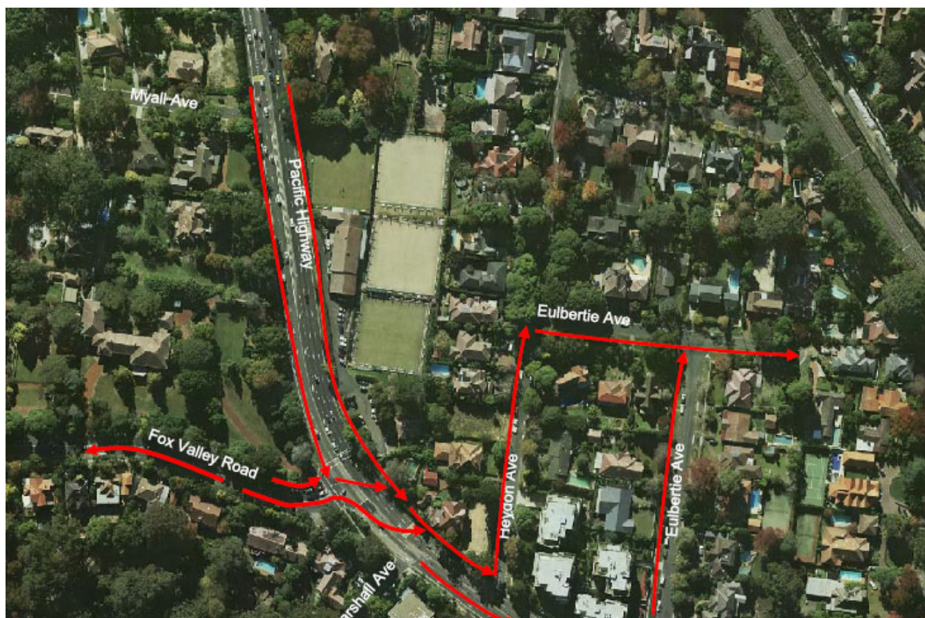
Figure 6-52: Existing stormwater flow direction through the proposal location at Intersection 2 (Roads and Maritime, 2018)
