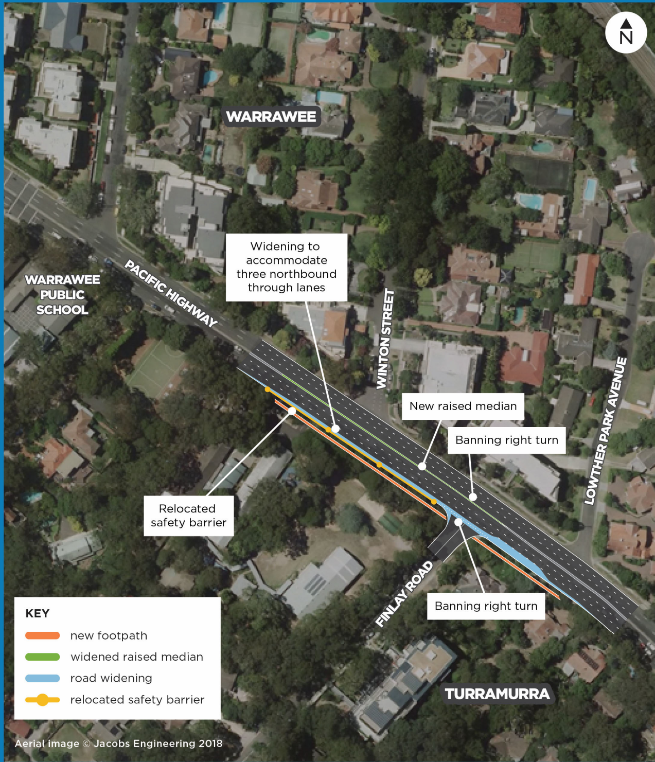
Figure 1-2: Main features of the proposal: Intersection 1 – Pacific Highway at Finlay Road, Warrawee/Turramurra
