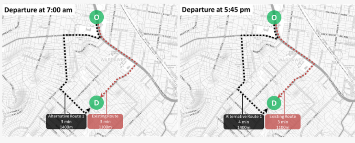
Figure 6-35: Proposed diversion routes as a result of the right-turn bans at Finlay Road, Warroo/Turramurra (excerpt from Route Diversion Assessment, Roads and Maritime, 2018)
