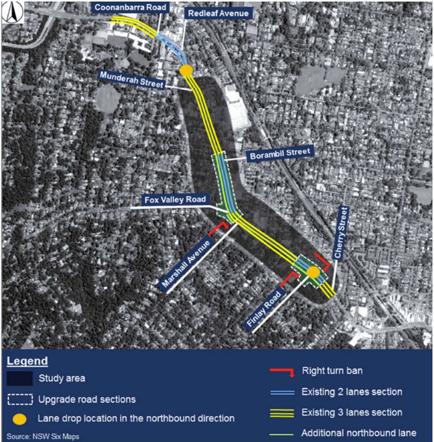
Figure 6-33: Location of lane number variability in the northbound direction between Turramurra and Wahroonga (excerpt from Traffic Performance Assessment - Roads and Maritime, 2019b)
