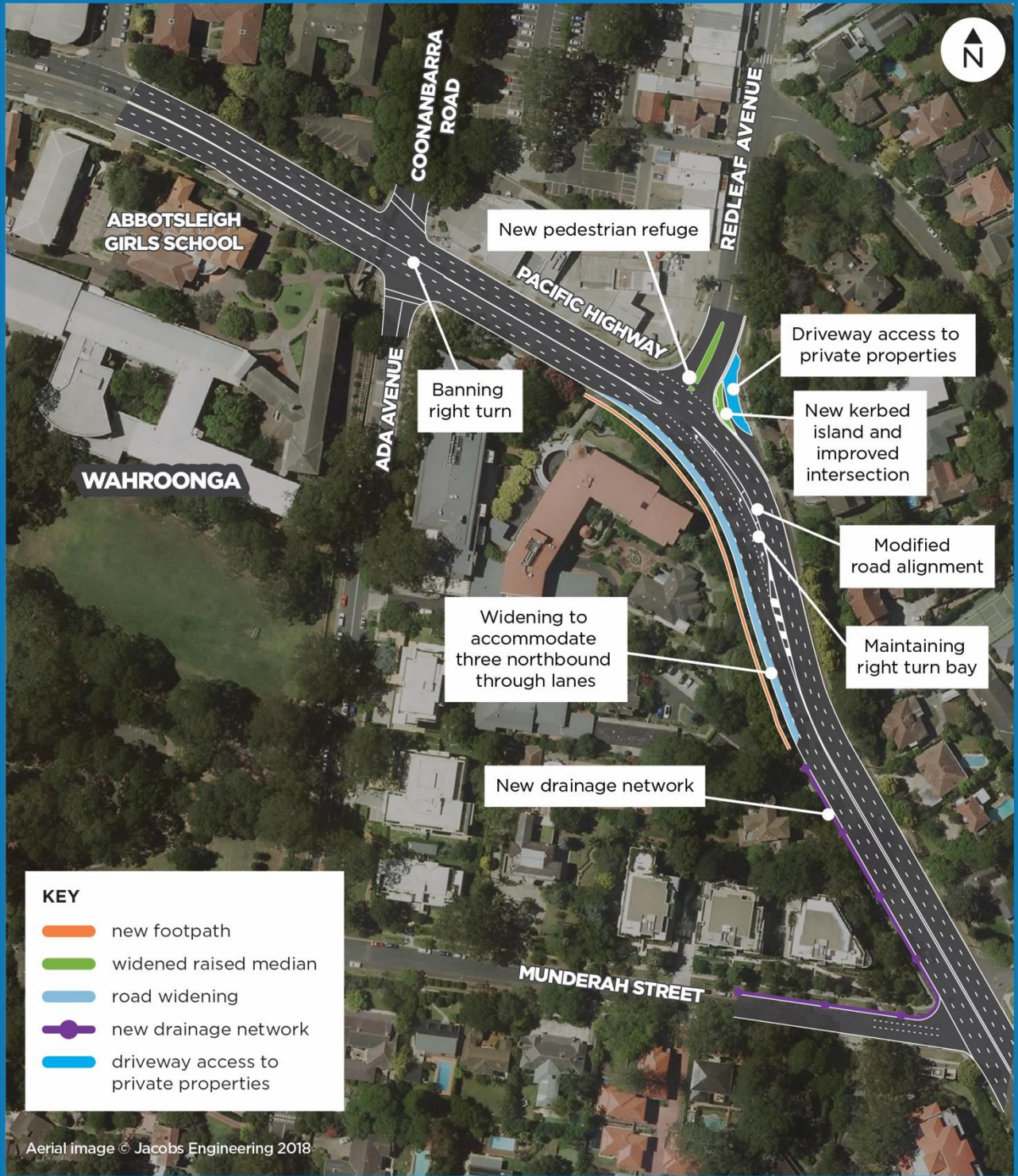
Figure 4: Proposed intersection upgrades on Pacific Highway at Coonanbarra Road and Redleaf Avenue
