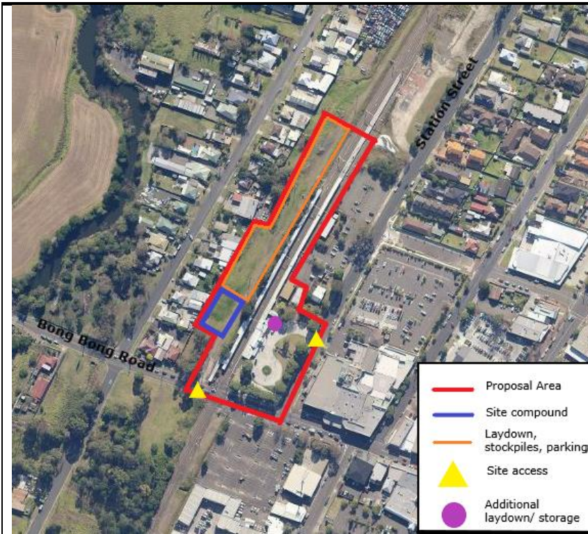
Figure 2: Dapto Station aerial photograph showing the indicative Project Area and site compound location
