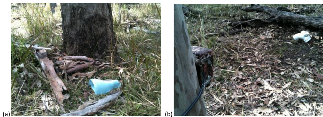
Plate 5: Hair funnels (a) and IR cameras aimed at bait stations (b) were used during baseline surveys of habitat surrounding the three monitored fauna culverts.
